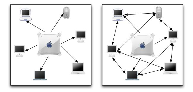
Figure 1: Client-Server (left) vs. Peer-To-Peer (right)
